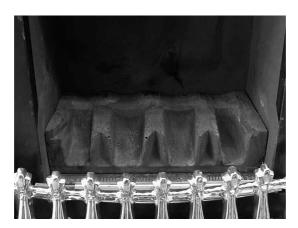
b) Position front ceramic rail on burner front ceramic support and ensure that the locating channel in the front ceramic rail is correctly located onto the lip on the burner front ceramic support. (See fig. 2 below)
