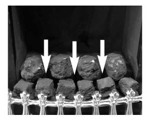
e) Select four of the medium coals and arrange along the rear of the fuelbed, using the recesses in the rear of the fuelbed as a guide for placement. (See fig. 5 below)
